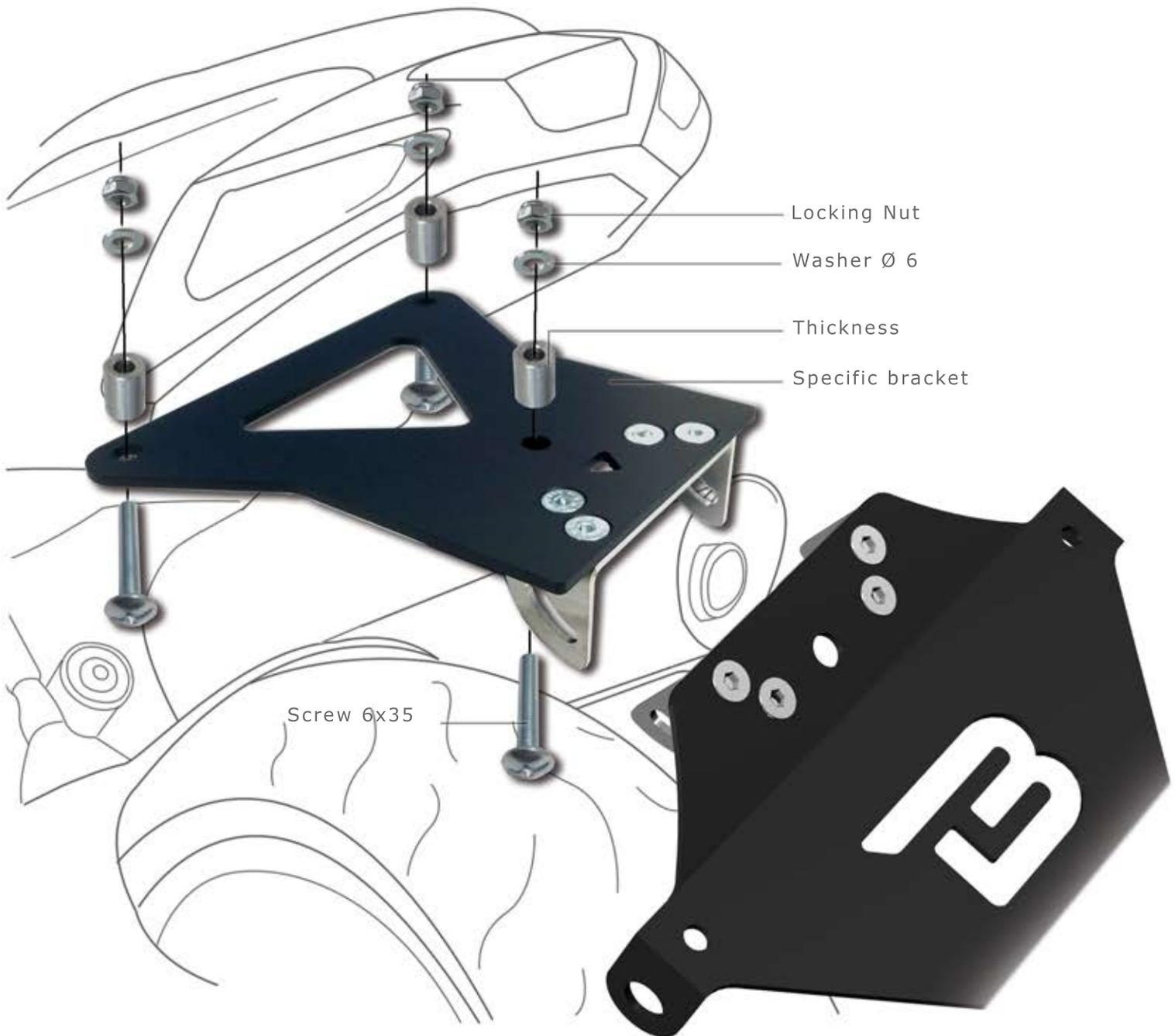
REMOVE THE ORIGINAL LICENCE PLATE FROM THE MOTORBIKE. APPLY THE BARRACUDA SPECIFIC BRACKET USING THE THICKNESS E AND SCREWS INCLUDED LIKE SHOWN IN THE PICTURE. APPROACH AND LOCK THE "X" LICENCE PLATE.
