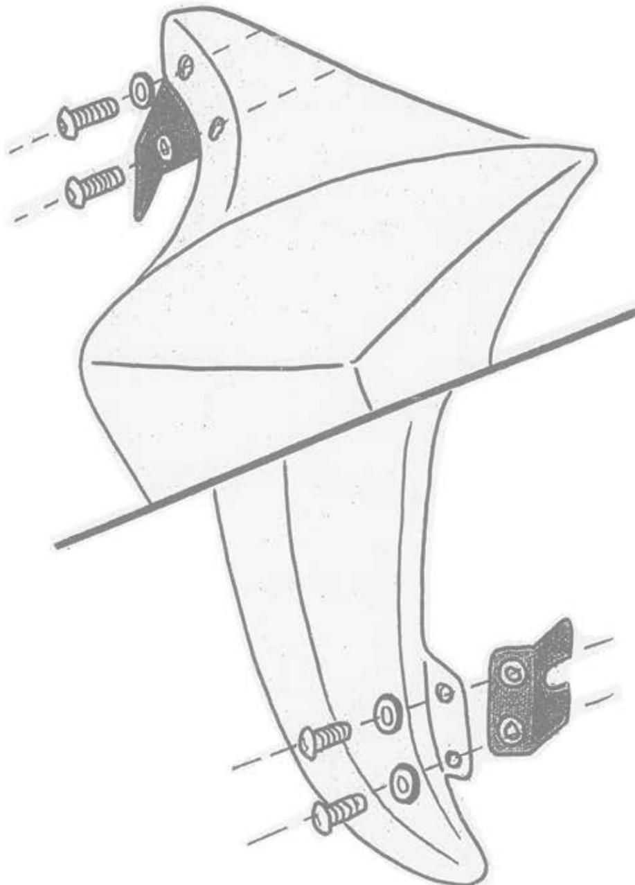
MOUNT THE BRACKETS ON THE BARRACUDA AIR CONTROL LIKE IN THE PICTURE. FIX THE BARRACUDA AIR CONTROL ON THE MOTORBIKE USING THE ORIGINAL SCREW IN THE UPPER PART OF RADIATOR AND THE 8X16 SCREW IN THE DOWN PART THE RESPECTIVE NUT.
